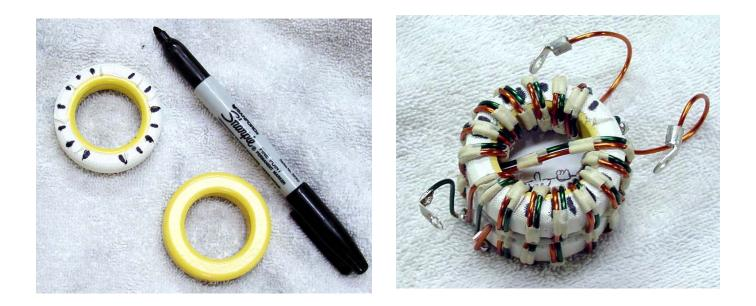
A thin cardboard spacer between the two cores will prevent damage to the magnet wire insulation. I used a separator from a 36 pack soft drink carton; cardboard from the back of a writing tablet is fine as well.
