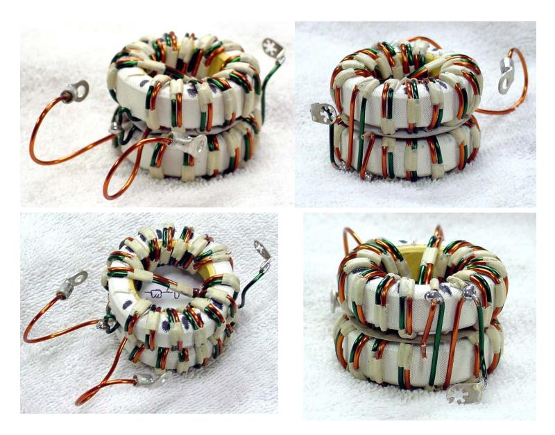
When clearance is required for scrapping insulation off a wire, gently bend/move the other wire out of the way - and remember to use smooth or rounded nose pliers. If you do not have smooth jaw pliers wrapping the tips with a few layers of tape will help to prevent nicking the insulation when forming the wires. Holding the core just above the project box will help you judge the positioning, length, and forming of the wires.
