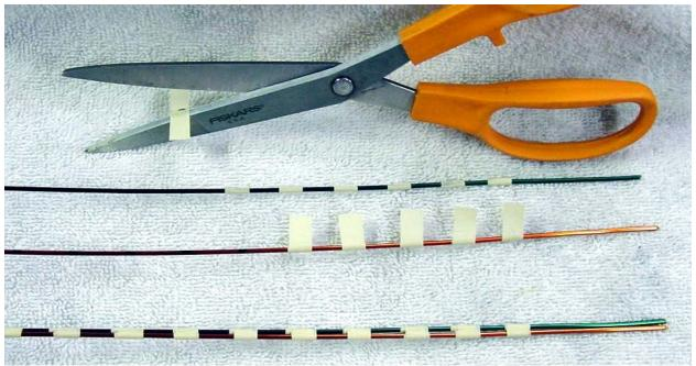
To prepare the transmission lines we start with 40 inches of wire. Starting 2 inches from one end apply the *spacing tape* for 31 inches on 3/4 centers.
