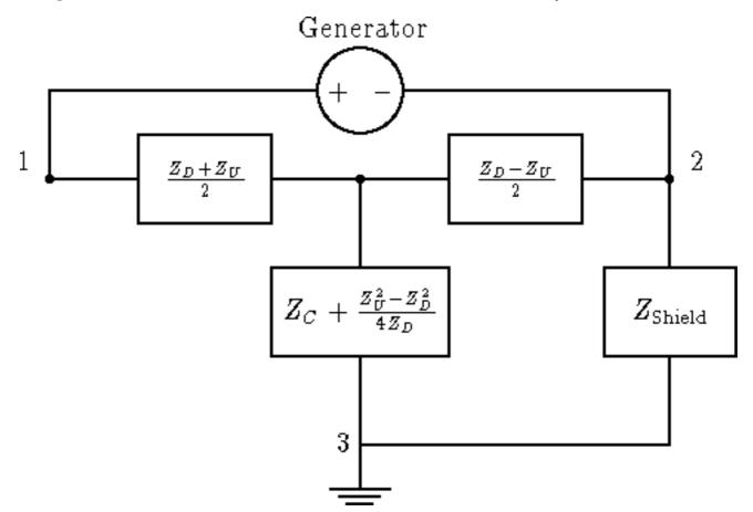
Figure 5: The W2DU model of coaxial cable connected directly to a balanced line.
