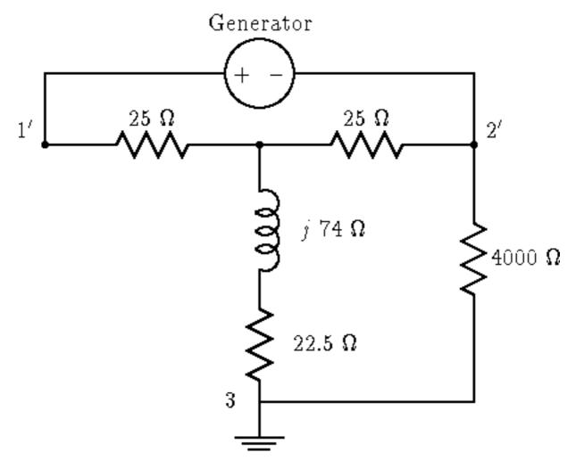
The new differential mode impedance is 50 ohms. The new common mode impedance is the old value plus the impedance of the two parallel inductors = 35 + j 74 ohms.
