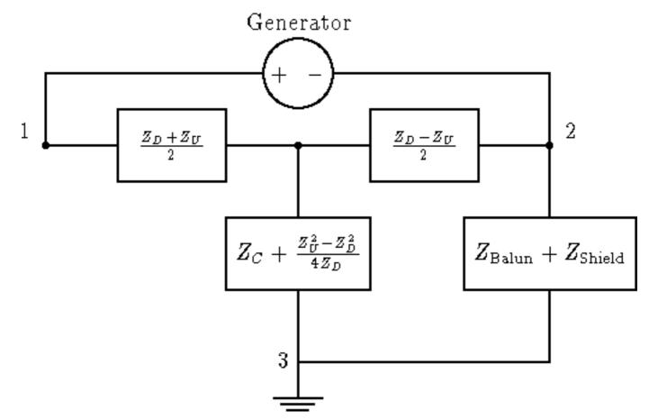
Maxwell's analysis gives a simple rule for understanding a choke balun connected to the three terminal network given by our twinlead fed antenna. Simply connect the balun common mode impedance from the terminal 2 to 3, and drive the antenna across terminals 1 and 2. If the current through terminal 3 is made small enough by the balun impedance, then the drive current is balanced between terminals 1 and 2.
