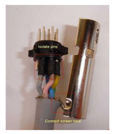
Cables should be shielded connecting grounds to the screens at the one side only to avoid ground loops.
