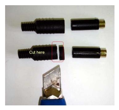
Soldering this connector is a real trouble... Do not use temperature over 250 C. **Be careful with +13.8V pin! Try to isolate it.**
