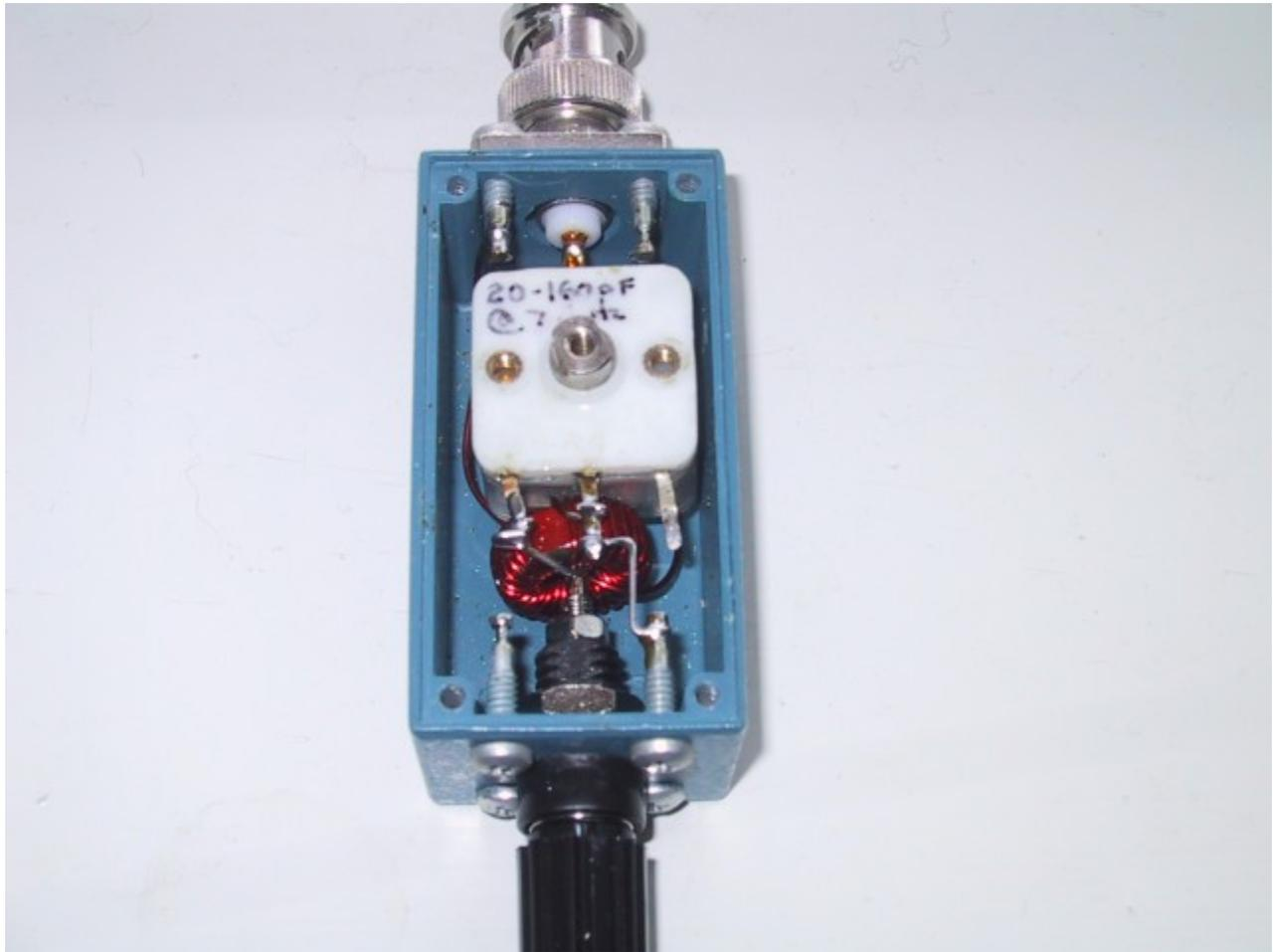
40m through 17m End Fed Half Wave Antenna Coupler built by AA5TB
