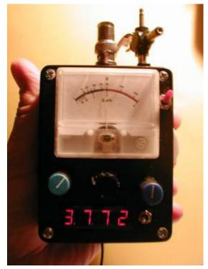
The completed "Mk1" antenna analyser
