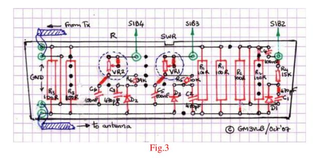
VR1 and VR2 are shown "dotted" as the exact placing of these components will depend on their shape, physical size and pin payout. The edges of the board are tapered as the ABS plastic boxes used are themselves tapered. This board slots into the "guides" at each side of the box. The dimensions of this board are approximately 2.9" (tapering to 2.8") by 0.8"
