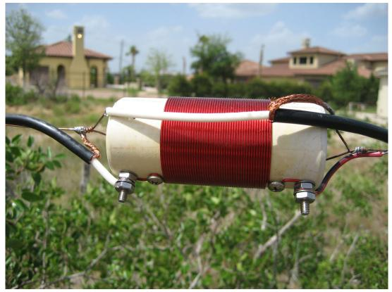
The ends of the coax capacitors need to have good voltage handling capability and be covered with rubber or silicone grease.
