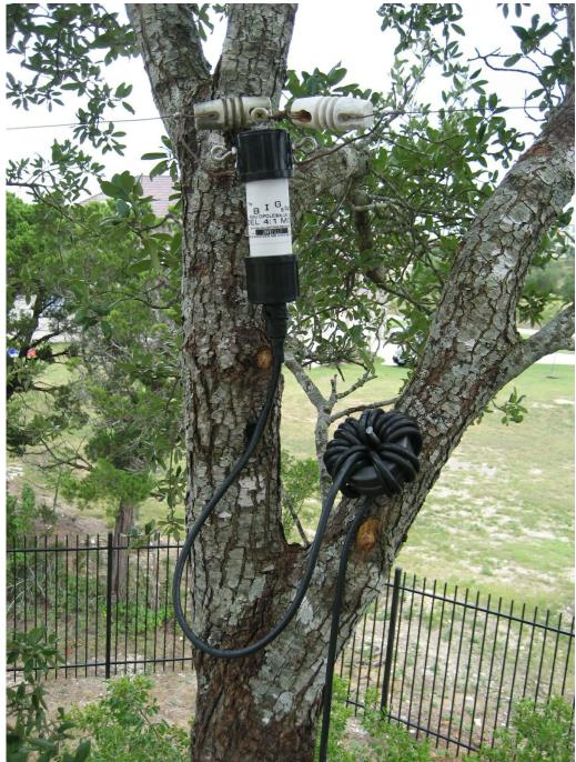
The 1:1 balun is 18 turns of RG8x on two 2.4 inch ferrite cores, type 43 or 77 material.
