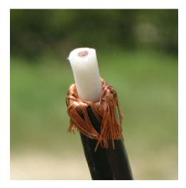
Here is the 55 uH inductor and coax capacitors "supported" with  $\sim$ 13' of plastic pipe sprayed camouflage green to help hide it.
