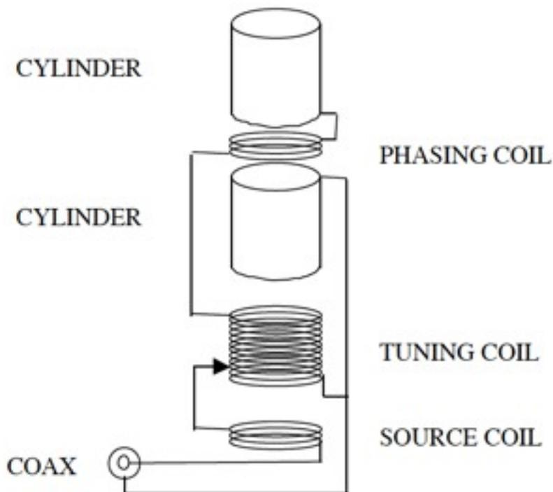
There are numerous links on the web providing information on the design, which I don't intend to repeat here. It suffices to say I am keenly interested in small antennas. I have made what I believe to be a thorough investigation of the EH antenna, of which this forms a part. This study is intended to prove, or disprove the existence of the phase shift between the fields.
