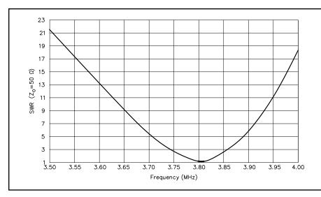
Fig 15—SWR versus frequency for voltage-fed half-square antenna, using matching network shown in Fig 10B, with L = 15  $\mu$ H, C<sub>1</sub> = 125 pF and C<sub>2</sub> = 855 pF. The SWR bandwidth is less than 100 kHz at the 2:1 SWR points.
