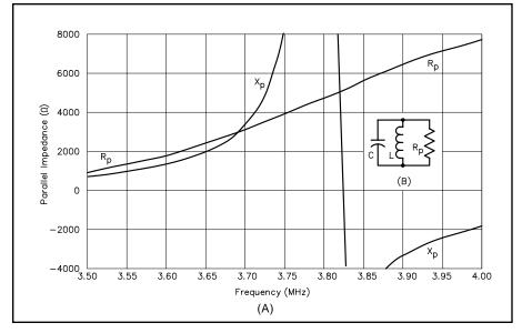
Fig 9—At A, graph of feed point shunt resistance and shunt reactance versus frequency for a half-square with voltage-feed at bottom corner. At B, equivalent parallel circuit of this antenna. This particular half-square is resonant at about 3.820 MHz, where its feed point resistance is about 5000  $\Omega$ .
