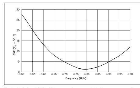
Fig 13—Variation of SWR with frequency for current-fed half-square antenna. The SWR bandwidth is quite narrow.
