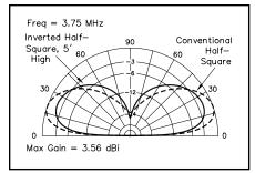
Fig 18—Elevation pattern for a conventional half-square, compared with an "inverted half-square" whose horizontal wire is located 5 feet over average ground. The difference is more than 2 dB.
