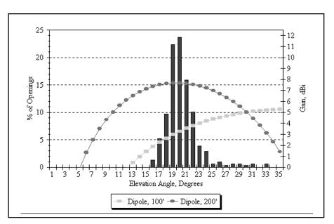
Fig 1—80-meter graph of the percentage of all openings from New England to Europe versus elevation angles, together with overlay of elevation patterns over flat ground for dipoles at two different heights. The 200-foot high dipole clearly covers the necessary elevation angles better than does the 100-foot high dipole. (*From The ARRL Antenna Book, 17th edition, Fig 30.*)
