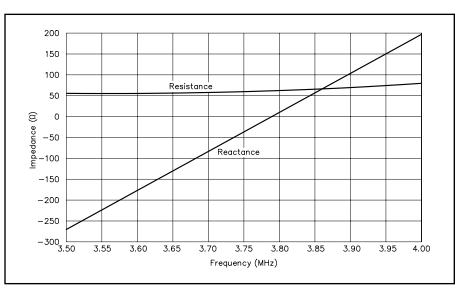
Fig 12—Graph of feed point series resistance and reactance versus frequency for a half-square with current-feed at one corner. Note that the resistive component changes slowly with frequency. This particular antenna is resonant at just under 3.8 MHz.
