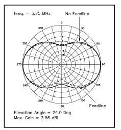
Fig 14—Effect of feed line on azimuth radiation pattern for current-fed halfsquare antenna. The feed line introduces only small distortions in symmetrical radiation pattern. The coaxial feed line was modeled as being brought out straight for 30 feet from the corner, then brought down close to ground level and led away for 50 feet more, where it was grounded.
