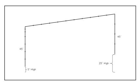
Fig 7—An asymmetrical distortion of the half-square antenna, where the bottom of one leg is purposely made 20 feet higher than the other. This type of distortion does affect the pattern!
