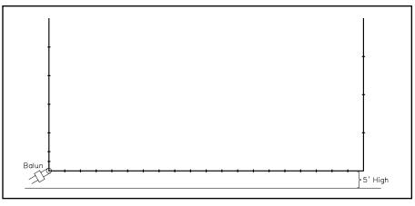
Fig 17—An "inverted half-square" antenna, current-fed at a lower corner. The losses in this configuration are excessive unless the ground under the antenna is exceptionally good, RF-wise.
