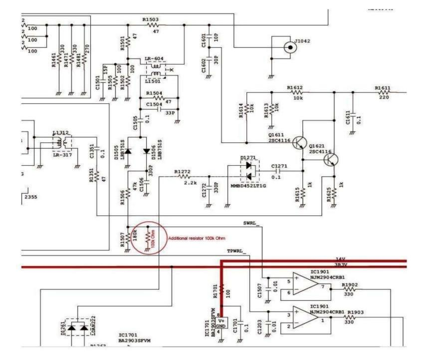
The best – experimentally found – value of the additional resistor is 100k Ohm. This value provides the practical matching range approx. SWR 1:6 (antenna impedance 8 to 300 ohm), that is much broader that originally.
