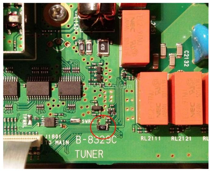
To do this mod, you have to remove the bottom cover of the radio and locate the resistor R1507 on the TUNER UNIT. It is just above in the middle of the PCB. A soldering iron for SMD parts with a fine tip is needed to solder precisely to the resistor's lead.
