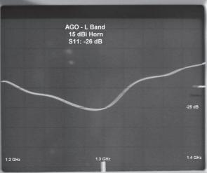
Appendances: Optimum 15 dBi pyramidal standard gain horn using smaller rectangular (2.6 x 5.6) waveguide, which cutoff is around 1.1 GHz (TE10). 6061 Al all wielded construction. This waveguide size (6 inches long) as shown above provided one of the better broad band return loss of the transitions tested. This illustrates that a variety of waveguide sizes from 5.6 to 8 inches wide can be tuned to work all measured better than -18 dB return loss.
