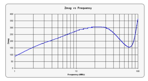
Next the output impdedance with the input terminated in a 50 ohm load.
