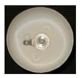
The connector is then soldered to the transformer, which is inserted inside the main part of the bottle. The inverted bottom section can then be pushed inside the base of the main section. This creates a waterproof seal, with a 50mm overhang which acts a rain shield around the connector.
