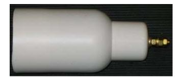
The finished unit can be secured to the supporting mast with tie-wraps. Two around the bottle, and one around the coax going into the base. This prevents the whole assembly from slipping down the mast.
