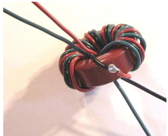
connector on the SO-239 already installed in the enclosure. Strip remaining green wire end 3/8" and bend into a hook for connection to the SO-239 ground connector.
