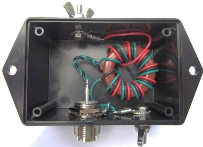
Position the toroid inside the box to allow connection of the red antenna wire lug to an 832 machine screw and lock-washer on the upper box side. Place a flat washer on the outside of the box followed with a # 8 lock washer/nut. Tighten the nut securely. Next, place the wing nut on the **antenna connector** and your project appears as shown above.
