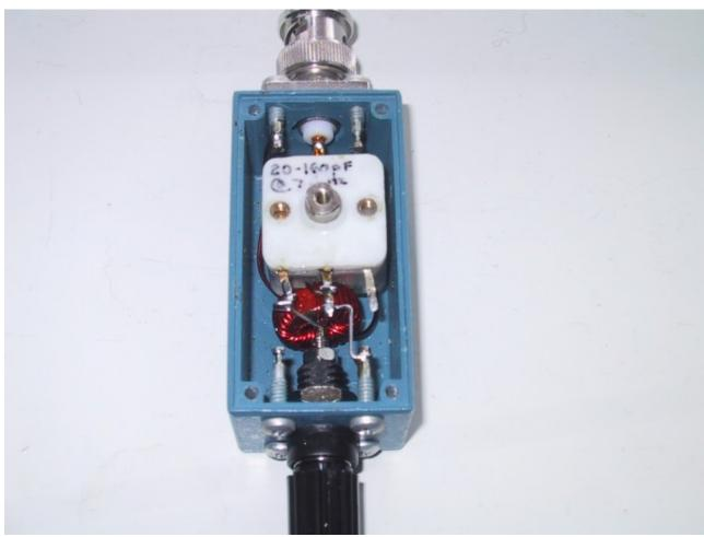
40m through 17m End Fed Half Wave Antenna Coupler built by AA5TB
