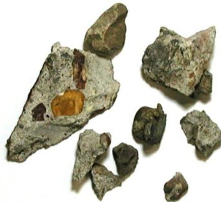
Figure 23. Concrete fragments from footer of foundation. Slab was undamaged, but the over-pour had these fragments blown off - from near the ground rod in Figure 10b.
