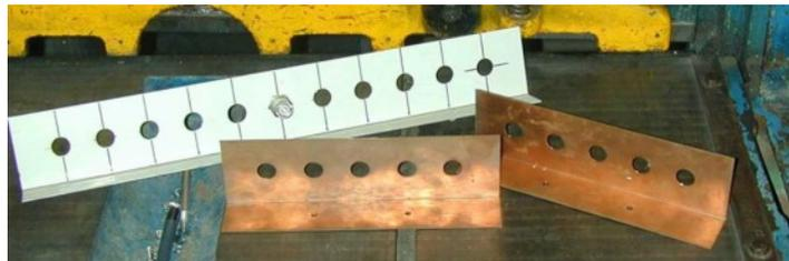
Figure 18. Shop made bulk head panels for single point grounding of incoming feed-lines. Picture from W8JI, [www.w8ji.com](http://www.w8ji.com).
