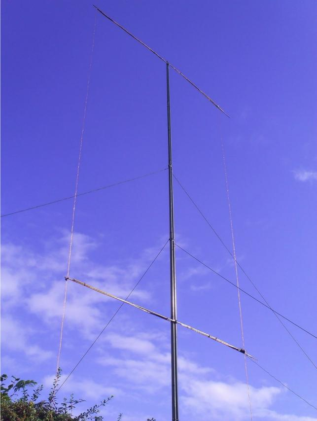
The central mast consists of two 9 metre fibreglass fishing poles, tie-wrapped together for extra rigidity, and fixed into the ground via two PVC wastepipe sections set into the lawn.
