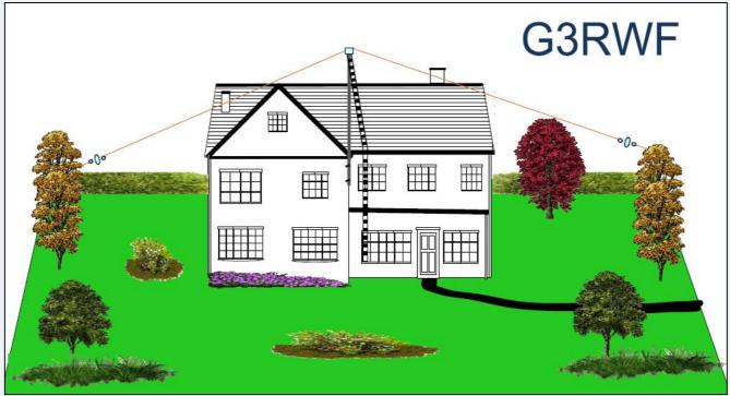
My antenna is at about 57 feet (17.4m) and the feeder is about 60ft (18.3m) long- almost vertical but comes into the house about 3 ft above ground level using commercial feed made from copper clad steel to an antenna matching unit (Palstar AT1KM) Nick R3RWF
