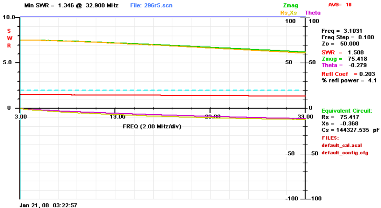
Dual 50-Ferrite Bead (#73)/RG-62 4:1 Balun: Load 296.5 Ohms
