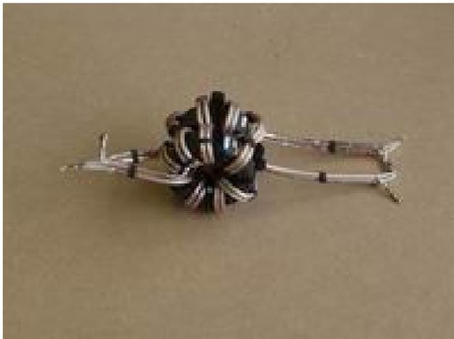
Now bind the two 1:1 Chokes together - again, I used a couple of plastic tie-wraps. Ensure that the two Chokes are aligned - i.e. the coaxes emerge at roughly the same positions
