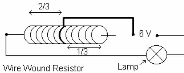
If the total resistance of the carbon track is 30 K $\Omega$  then the resistance between the wiper and the top connection would be 10 k $\Omega$ . If The wiper is moved to the top and then the bottom the resistance would be 0 Ohms ( Short circuit ) and 30 K $\Omega$  respectively.
