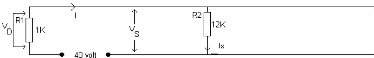
First find the resultant resistance ( Rt ) of the two resistors in parallel:
