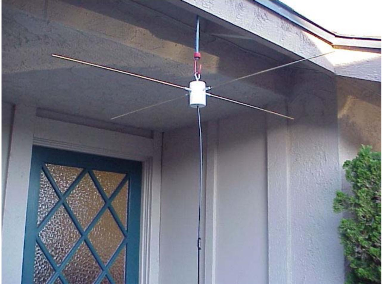
I came up with this antenna design for use with hidden transmitters on international-rules ARDF events. The rules call for an omnidirectional horizontally-polarized transmitting antenna at a height of two to three meters above ground level. Here in Southern California we have typically used vertical polarization in the past. This same antenna could be used for satellite or space communications as well with the addition of an appropriate reflector.
