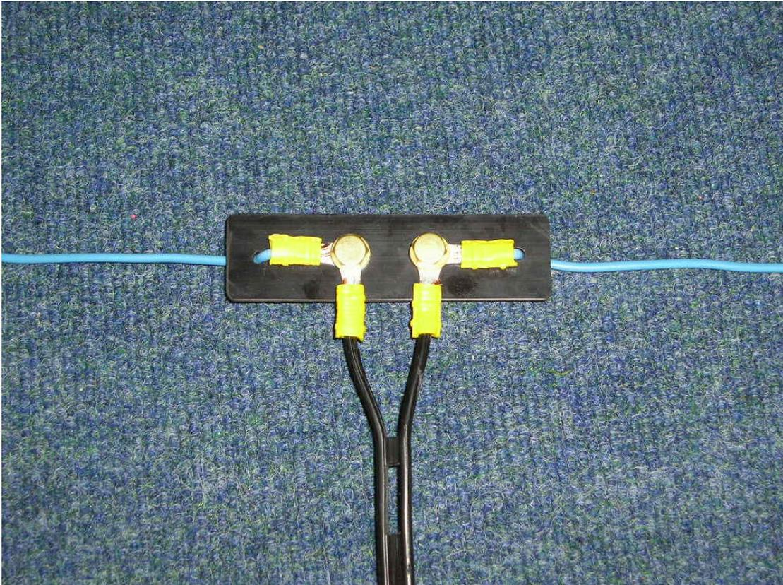
You will see from the above picture the assembly of the top section [blue wire] Each 31.05 M [102 Feet] length of blue wire is terminated with a 6MM Yellow crimp. Make sure it is soldered as well as crimped on **AFTER** you have passed it through the centre insulator. The purists amongst you will undoubtedly have noticed a slight design flaw in that the wire passes through the insulator and may be a weak point in the wind as the antenna sways around.
