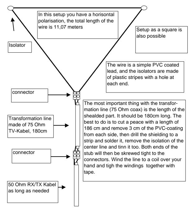
I put up the antenna in the loft, the antenna worked well from the beginning. Dipending on the surroundings you might have to tune it, by changing the length of the radiating wire. I worked a lot of stations with this antenna!
