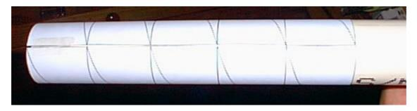
• The end you start the template at will be the end that connects to the base. Note, you should start protruding about the thickness of the endcap over the edge. See diagram below. This will compe thickness of the 40mm endcap
