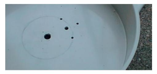
• Take the 40mm PVC endcap and cut off a section big enough to allow the N connector stub and tl to poke through. The sketch below will give you an idea of how much you want to cut off to allo bolt holes to fit when it all comes together.
