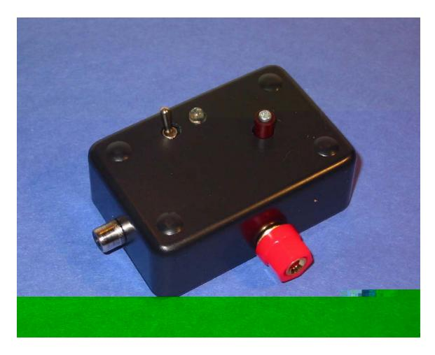
This kit was designed for use by travelers, packers, and other ultra/P amateur operators needing a lightweight, easy to deploy antenna system. Using this tuner, a portable station needs no ground radials and little or no feedline to achieve excellent results. Special attention has been paid to packability, durability, and reliability of operation. The tuner matches the impedance of end fed, half wavelength wires on the 40 through 15 meter amateur bands, and contains a built in SWR indicator.
