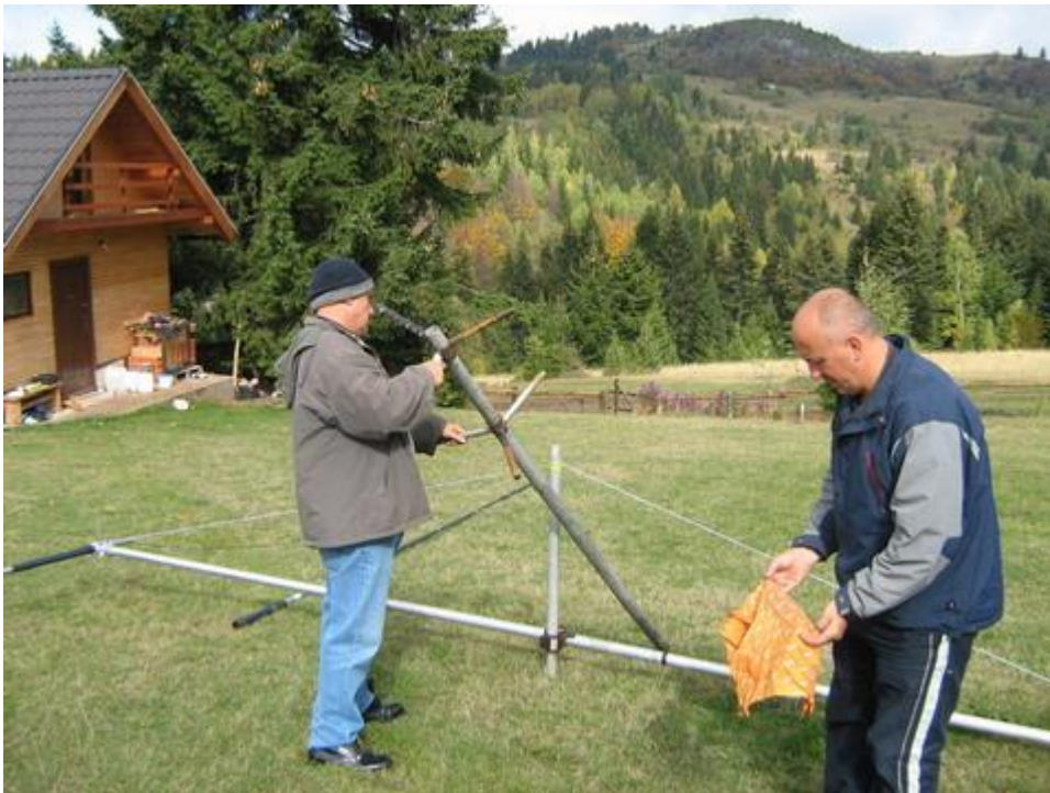
Andra (left) and Tafro working on the 40 meter moxon
