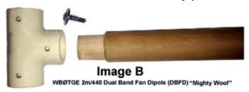
Looking at Image B, drill three 1/8" pilot holes on one side of the plastic tee about 1/4" from the ends of the openings. The image shows the 1/2" self-tapping screw used and the hardwood dowel used as the the mounting mast for the antenna. Sand the dowel end to match the inside diameter of the tee. Make it a press fit and long enough to seat completely into the tee opening. The copper pipes and wood dowel are secured to the tee using the self-tapping screws.
