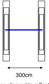
Driven element to reflector spacing on all bands
