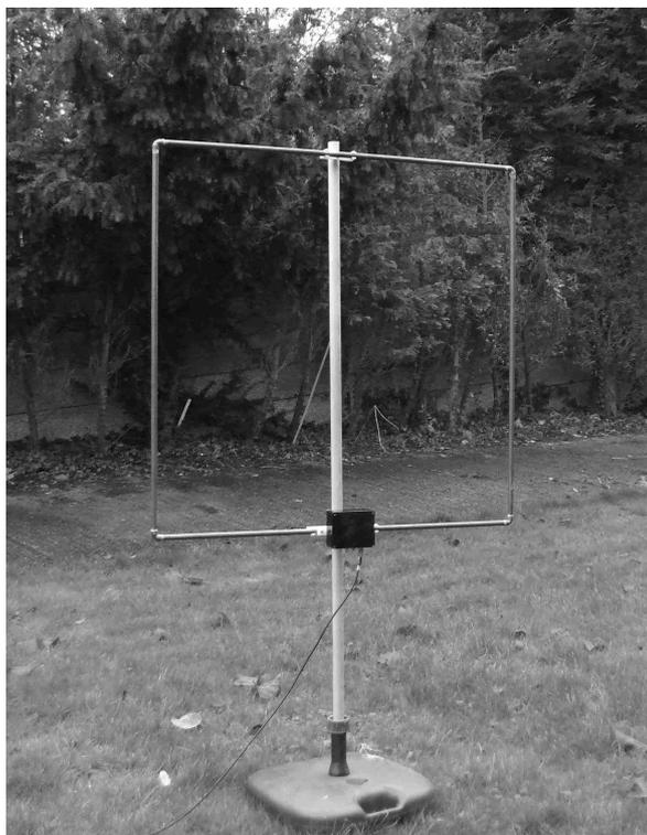
Figure 1 – 1m<sup>2</sup> bandpass loop antenna
