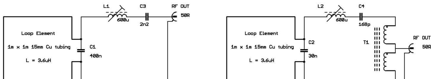
Figure 2 (a)  $136\text{kHz}$ , (b)  $500\text{kHz}$  loop circuits
