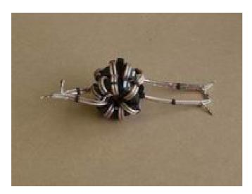
Now bind the two 1:1 Chokes together - again, I used a couple of plastic tie-wraps. Ensure that the two Chokes are aligned - i.e. the coaxes emerge at roughly the same positions
