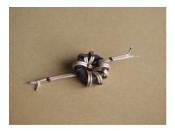
Now wind 8 turns of this twin cable onto a FT140-61 toroid to form a 1:1 Choke. The "crossover" winding is not an electrical requirement - it's just an easy way to get the coaxes to emerge at opposite ends of the ferrite core. Use a couple of plastic tiewraps to hold the coax to the core at each end.
