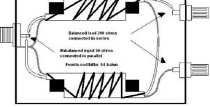
The Guanella 4:1 Current Balun tested with two 100 ohm resistors in series and an Antenna Analyser gave the following results
