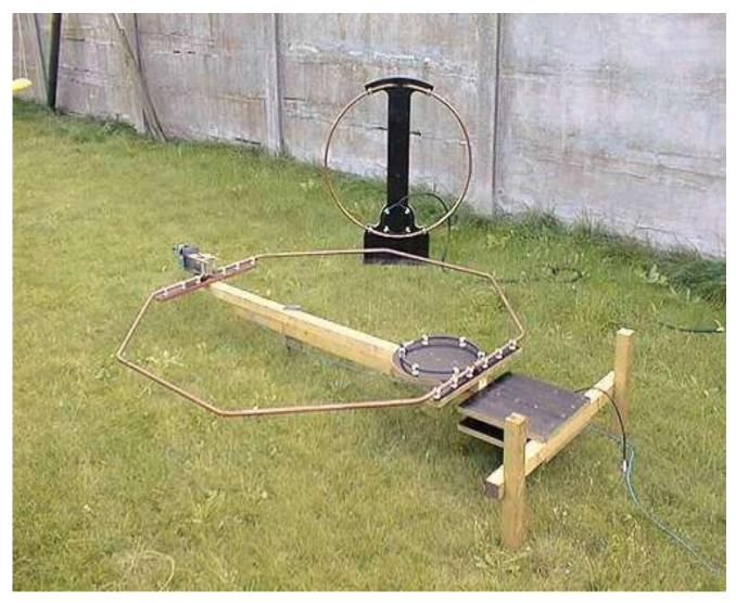
The first one turn loop that I built was made from 75 Ohm TV Coax and with a small explanation in the RSGB handbook for radio amateurs. I used the outer screen from the coax and the results of the loop where good. The next loop I built is a octagon loop in 15mm copper tube with a circumference of 4.8 meter (16 feet).
