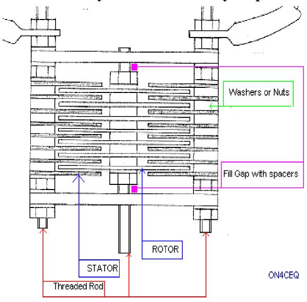
The best material for the front and the back is CLEAR PVC 3 or 5 mm thick as alternative you can use GREY PVC or 2 sheets pc board together with the copper removed.
