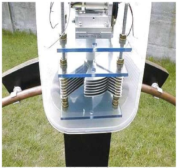
The second capacitor I built is my own design and it's a butterfly capacitor because the losses are lower than a split stator. The capacitance is 5-65 pF and the voltage rating is 7200 volts. I used it for the small loop with a dia. of 800 mm (2.66 feet) and the frequency range of this loop is from 28 MHz to 14 MHz. The Aluminum plates of 1 mm for the capacitors are cut with a JIG SAW
