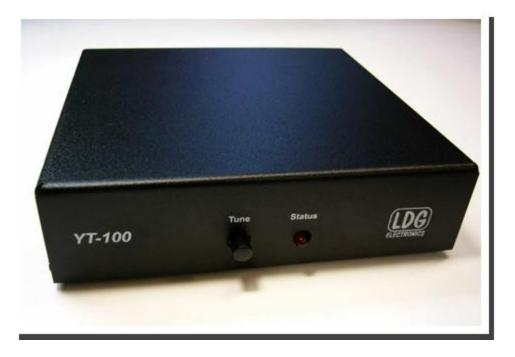
**Tune Button:** Initiates either a memory tune or a full tune, and also toggles the tuner between "active" and "bypass" modes.
