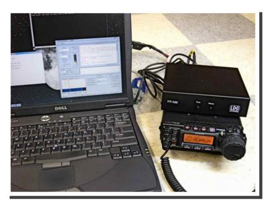
The YT-100 monitors the **Computer** port for activity before beginning any tuning cycle. Only when the CAT line is idle for a period of time will the YT-100 take over control of the CAT line in order to
