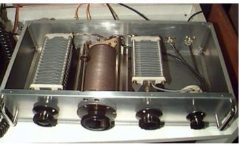
three wafers each having five way switching (3 x single pole, 5 way) on a common shaft will allow selection of two separate antennas (A or B) in a bypass or through ATU situation, plus a spare contact for a dummy load or off position.
