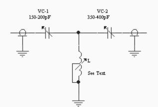
The Simple but effective T-Network type ATU Tri-pole, 5 way switching was added for ant A, B or Dummy. - A High Voltage ceramic insulated single pole multi-way switch is used to short the unused turns to ground.
