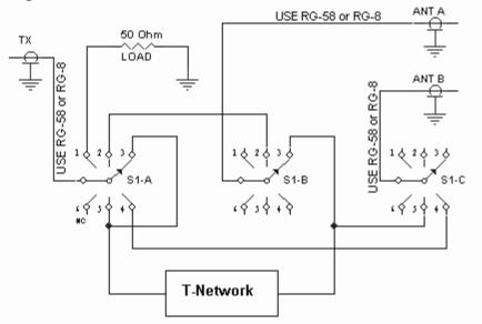
If you wish to add antenna or dummy load switching as I did, then you must run 50 Ohm coax between all sockets and switches. The coaxial braid must be earthed at any sockets and joined at all break points around switch gear, this will minimise the introduction of Standing Waves when switched through (ATU by-passed). A set of
